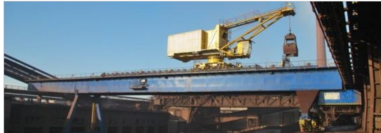
Full-portal gantry crane for bulk material handling, span of crane = 45 m, lifting capacity = 16 t
